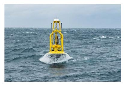
This latest deployment of a PB3 PowerBuoy<sup>®</sup> will serve Premier as an autonomous intelligent platform to provide communications and remote monitoring services at Premier's Huntington field in the central North Sea. During the deployment, Premier will demonstrate the PB3 PowerBuoy<sup>®</sup> capabilities, its ability to monitor the local environment and alert ships of the field's safety zone as a potential solution to help with their future decommissioning related operations.
