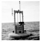
Our PowerBuoy system consists of a floating buoy-like device that is loosely moored to the seabed so that it can freely move up and down in response to the rising and falling of the waves, as well as a power take off device, an electrical generator, a power electronics system and our control system, all of which are sealed in the unit.
