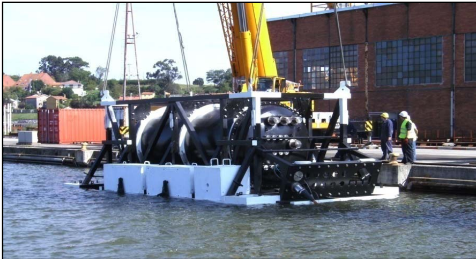
Undersea Substation Pod readied for deployment
