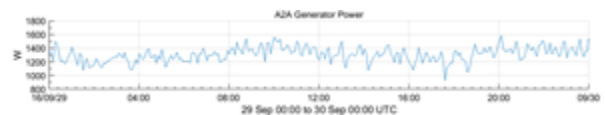
Example of the PB3 PowerBuoy daily power generation, as measured by its internal instrumentation over a 24-hour period in high sea-states (September 29th 2016). This, and other data is live-streamed to OPT headquarters in Pennington, NJ
