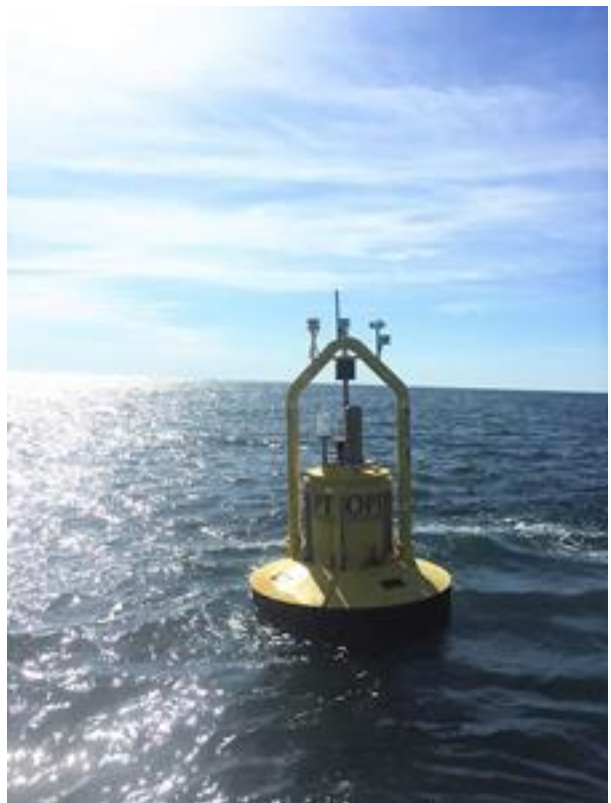
Deployed PB3 PowerBuoy off the coast of New Jersey
